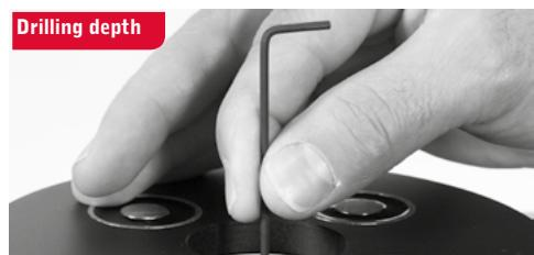
The drilling depth is preset ex works. The drilling depth is adjusted with the Allen key under the drill in the drilling axis with the aid of the provided mounting tool.
