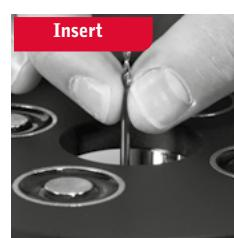
Always switch the unit off first and disconnect the mains plug. Loosen the two lateral grub screws in the drill spindle with the provided Allen key and pull out the drill. Insert the new drill and tighten both grub screws tightly and evenly. To set a new drilling depth, please proceed as described in section "Setting drilling depths". Switch the unit back on and perform test drilling.
