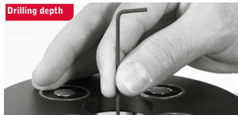
The drilling depth is preset ex works. The drilling depth is adjusted with the Allen key under the drill in the drilling axis with the aid of the provided mounting tool.
