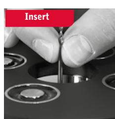
Always switch the unit off first and disconnect the mains plug. Loosen the two lateral grub screws in the drill spindle with the provided Allen key and pull out the drill. Insert the new drill and tighten both grub screws tightly and evenly. To set a new drilling depth, please proceed as described in section "Setting drilling depths". Switch the unit back on and perform test drilling.
